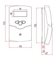
The DeltaSol<sup>®</sup> BS is a controller for standard solar thermal systems. It provides a clear operating concept and is equipped with a system-monitoring display. Flashing symbols for sensors, pumps and valves show temperatures, temperature differences and active actuators. The DeltaSol<sup>®</sup> BS controller is available in 4 versions
