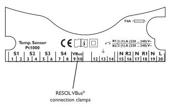
The controller comes with a RESOL **VBus**<sup>®</sup> for data communication and energy supply of external modules. The connection is effected with optional polarity at the clamps marked with,,VBus".Via this data Bus you can install one or more RESOL VBus<sup>®</sup> modules, e.g.:
